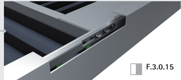
用滑轮导引内框架 Internal frame guided with castors.
